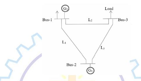
Obtain the load flow solution at the end of the first iteration of the power system shown in the figure. The data is provided in the Table. The solution is to be obtained for the following cases .
